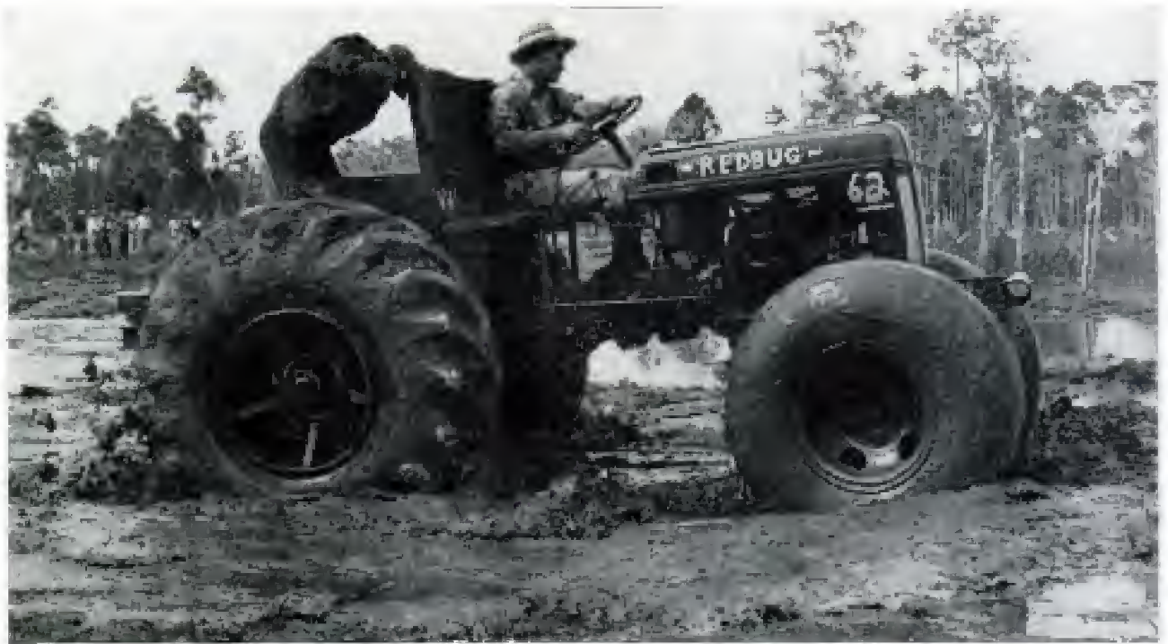
"Redbug," a revamped tractor, is geared for more speed but retains original power. Its tires need no chains
